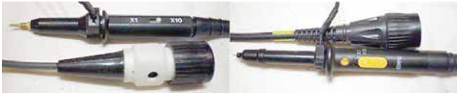
Fig.5: compensation trimmer at the scope end (left) and probe end (right).
