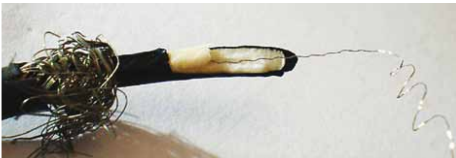
Fig.8: probe cable dissection – note the crinkled inner wire.
