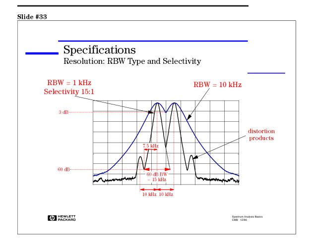
For example, say we are doing a two-tone test where the signals are separated by 10 kHz. With a 10 kHz RBW, resolution of the equal amplitude tones is not a problem, as we have seen. But the distortion products, which can be 50 dB down and 10 kHz away, could be buried.
