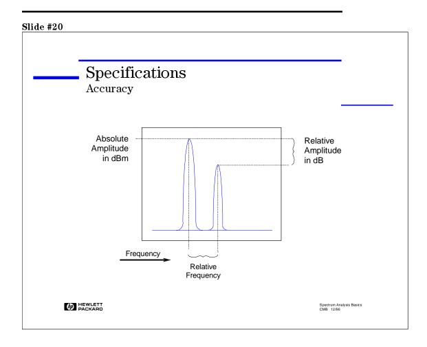
The second area to understand is **accuracy**; how accurate will my results be in both frequency and amplitude? When talking about accuracy specifications, it is important to understand that there is both an absolute accuracy specification, and a relative accuracy specification.
