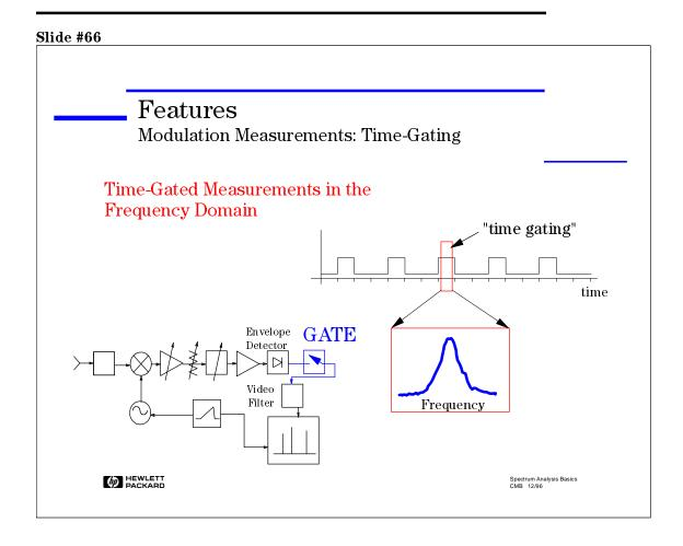
Time-gated, or time-selective spectrum analysis offers a solution to measurement difficulties in the time and frequency domains. Time gating permits precise yet flexible control of the point at which a time domain sweep begins, allowing the sweep to be centered over the desired timeslot. Any timeslot, or portion of a timeslot, may be examined at maximum time resolution.
