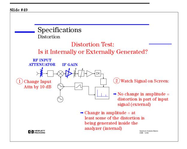
Before leaving this section on distortion, there is a test that should be done for all distortion measurements. The test is going to tell us whether or not what we are seeing on the screen is internally generated distortion, or distortion caused by the DUT.
