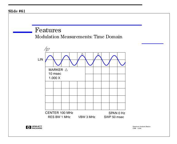
It was mentioned briefly that although a spectrum analyzer is primarily used to view signals in the frequency domain, it is also possible to use the spectrum analyzer to look at the time domain. This is done with a feature called zero-span. This is useful for determining modulation type or for demodulation.
