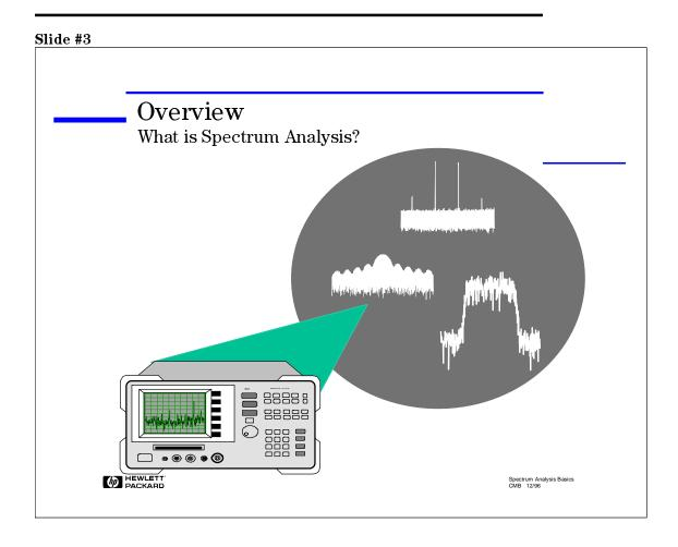
If you are designing, manufacturing, or doing field service/repair of electrical devices or systems, you need a tool that will help you analyze the electrical signals that are passing through or being transmitted by your system or device. By analyzing the characteristics of the signal once its gone through the device/system, you can determine the performance, find problems, troubleshoot, etc.
