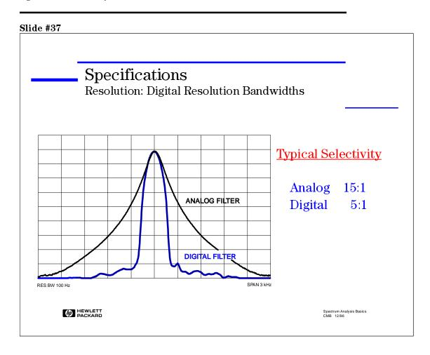
One thing to note before we close the topic of resolution is that Digital RBWs (i.e. spectrum analyzers using digital signal processing (DSP) based IF filters) have superior selectivity and measurement speed. The following table illustrates this point. For example, with a 100 Hz RBW, a digital filter is 3.1 times faster than an analog.
