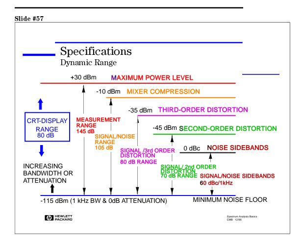
There are several ranges associated with the spectrum analyzer. Typically the term "dynamic range" only refers to the ability to measure two signals at the same time.
