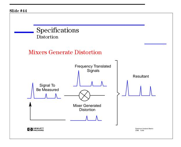
Although distortion measurements, such as third order intermodulation and harmonic distortion, are common measurements for characterizing devices, the spectrum analyzer itself will also produce distortion products, and potentially disturb your measurement.
