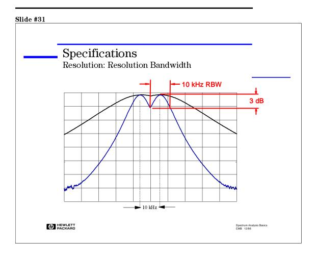
When measuring two signals of equal-amplitude, the value of the selected RBW tells us how close together they can be and still be distinguishable from one another (by a 3 dB 'dip'). For example, if two signals are 10 kHz apart, a 10 kHz RBW easily separates the responses. However, with wider RBWs, the two signals may appear as one.
