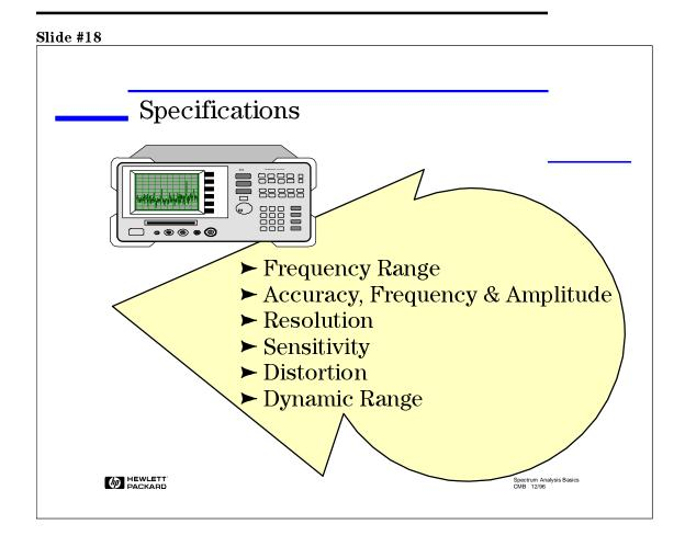
What do you need to know about a spectrum analyzer in order to make sure you choose one that will make your particular measurements, and make them adequately? Very basically, you need to know 1) what's the frequency range? 2) what's the amplitude range (maximum input and sensitivity)? 3) to what level can I measure the difference between two signals, both in amplitude (dynamic range) and frequency (resolution)? and 4) how accurate are my measurements once I've made them?
