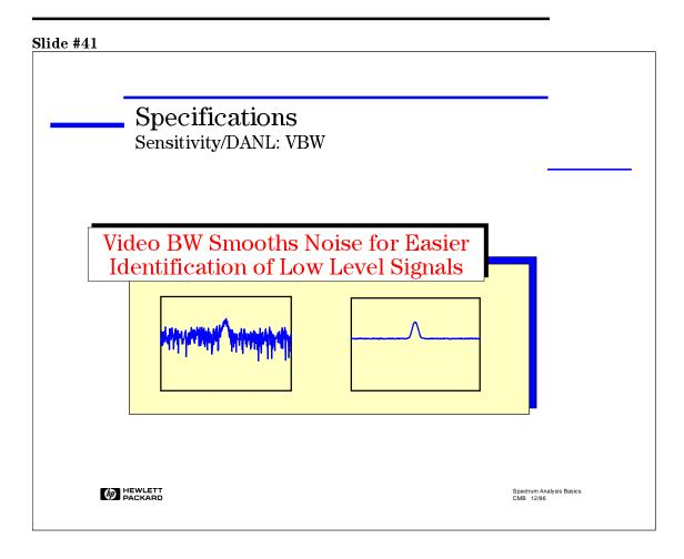
In the Theory of Operation section, we learned how the video filter can be used to smooth noise for easier identification of low level signals. Since we are talking about measuring low level signals, we will repeat it here. The VBW, however, does not effect the frequency resolution of the analyzer (as does the RBW), and therefore changing the VBW does not improve sensitivity. It does, however, improve discernability and repeatability of low signal-to-noise ratio measurements.
