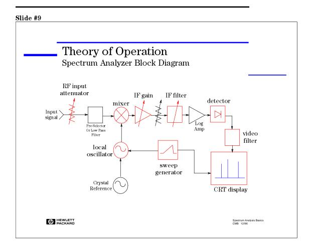
The major components in a spectrum analyzer are the RF input attenuator, mixer, IF (Intermediate Frequency) gain, IF filter, detector, video filter, local oscillator, sweep generator, and CRT display. Before we talk about how these pieces work together, let's get a fundamental understanding of each component individually.
