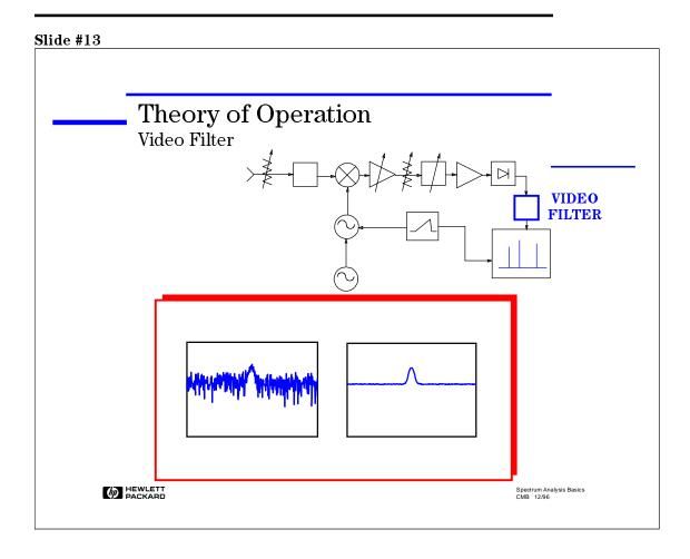
The video filter is a low-pass filter that is located after the envelope detector and before the ADC. This filter determines the bandwidth of the video amplifier, and is used to average or smooth the trace seen on the screen.
