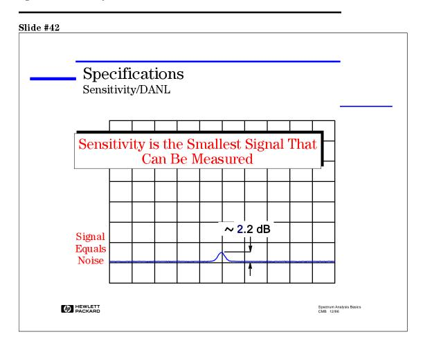
A signal whose level is equal to the displayed average noise level (DANL) will appear approximately as a 2.2 dB bump above the displayed average noise level. This is considered to be the minimum measurable signal level. However, you won't be able to see this signal unless you use video filtering to average the noise.
