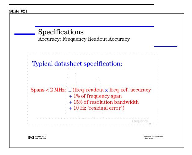
Frequency accuracy is often listed under the Frequency Readout Accuracy specification and is usually specified as the sum of several sources of errors, including frequency-reference inaccuracy, span error, and RBW center-frequency error.
