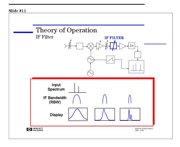
The IF filter is a bandpass filter which is used as the "window" for detecting signals. It's bandwidth is also called the resolution bandwidth (RBW) of the analyzer and can be changed via the front panel of the analyzer.
