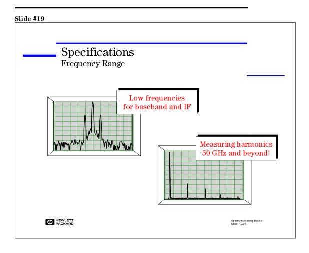
Of course, the first and foremost specification you want to know is the **frequency range** of the analyzer. Not only do you want a spectrum analyzer that will cover the fundamental frequencies of your application, but don't forget harmonics or spurious signals on the high end, or baseband and IF on the low end.
