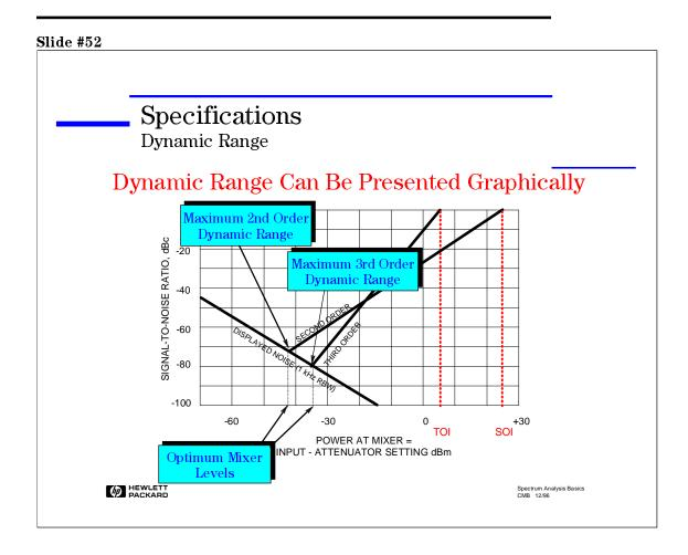
Let's plot both the signal-to-noise and signal-to-distortion curves on one dynamic range graph. *Maximum dynamic range* occurs where the curves intersect, that is, when the internally generated distortion level equals the displayed average noise level. This shows two of the dynamic range specifications. We will see that there are others later.
