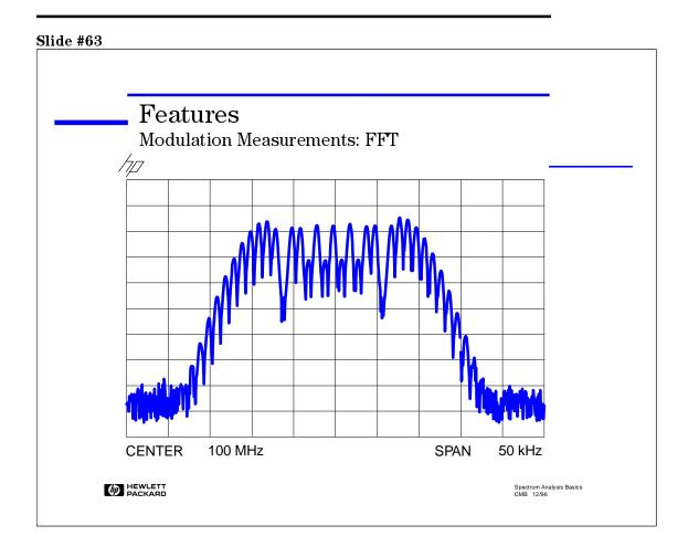
We've just seen how modulation frequency and AM depth of modulation measurements using a spectrum analyzer can be made in both the swept-frequency-domain and the FFT-frequency-domain. So why would you want to use the FFT function?
