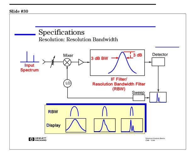
One of the first things to note is that a signal cannot be displayed as an infinitely narrow line. It has some width associated with it. This shape is the analyzer's tracing of its own IF filter shape as it tunes past a signal. Thus, if we change the filter bandwidth, we change the width of the displayed response. HP datasheets specify the 3 dB bandwidth. Some other manufacturers specify the 6 dB bandwidth.
