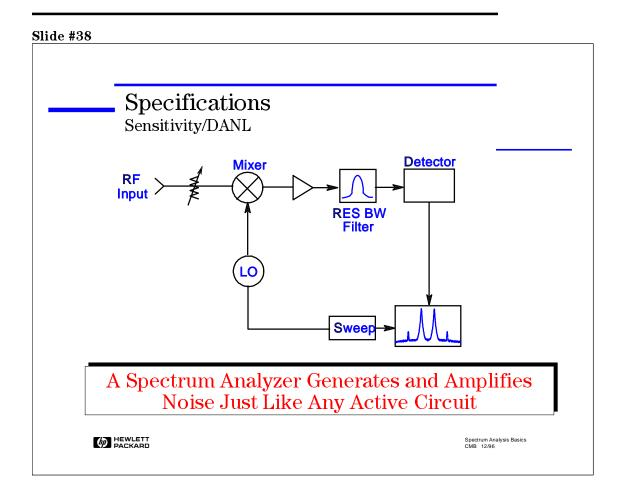
One of the primary uses of a spectrum analyzer is to search out and measure low-level signals. The **sensitivity** of any receiver is an indication of how well it can measure small signals. A perfect receiver would add no additional noise to the natural amount of thermal noise present in all electronic systems, represented by kTB (k=Boltzman's constant, T=temperature, and B=bandwidth). In practice, all receivers, including spectrum analyzers, add some amount of internally generated noise.
