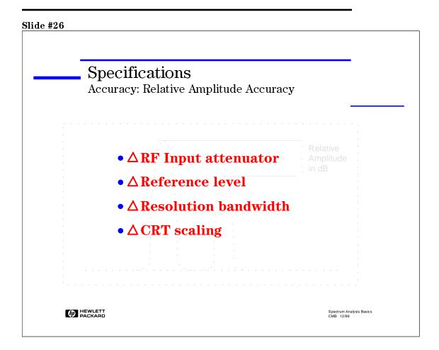
As we mentioned before, the four items listed above involve control changes made during the course of a measurement, and can be eliminated if they can be left unchanged.
