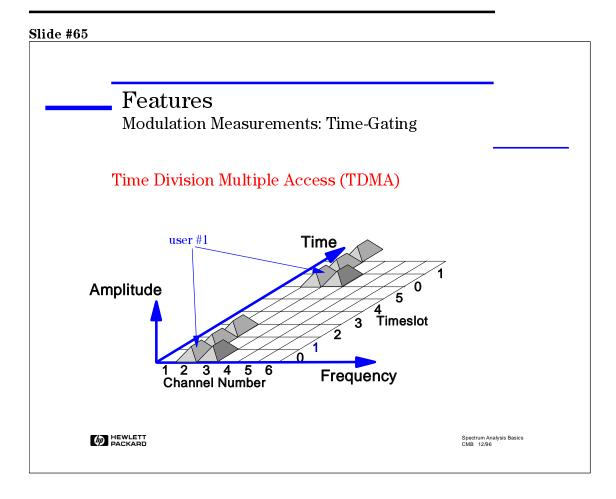
In order to explain the time-gating feature of a spectrum analyzer, we will use a digital communications application, Time-Division-Multiple-Access (TDMA). This is a common method used in communications in order to increase channel capacities in the same frequency bands. TDMA divides up the frequency channels into time slots, so that users can occupy the same frequency, but use different timeslots.
