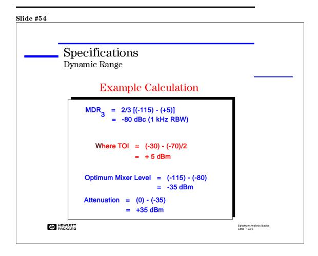
For example, let's say we have a spectrum analyzer with a DANL = -115 dBm  $\,(1~\rm kHz~RBW)$ , and TOI = +5 dBm. This slide shows how to calculate maximum third-order dynamic range  $\,(MDR_3)$ , optimum mixer level, and attenuation.
