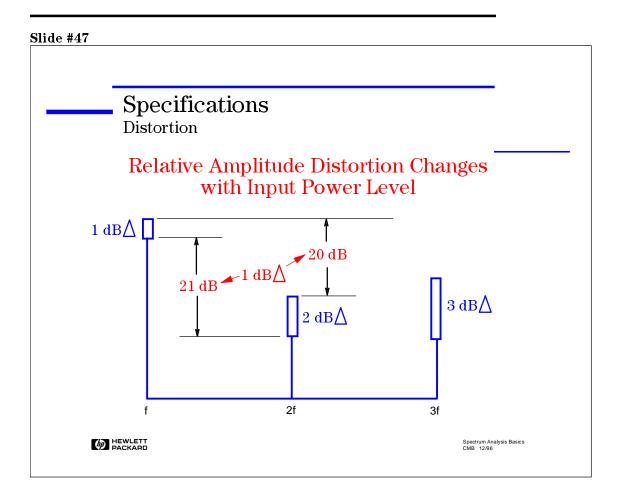
Most distortion measurements are made relative to the fundamental signals (the carrier or two-tones). When the fundamental power is decreased 1 dB, the second-order distortion decreases by 2 dB, but relative to the fundamental, the second-order distortion decreases 1 dB. There is a one-for-one <u>relative</u> relationship between the fundamental and second-order distortion.
