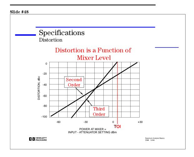
Understanding this concept is useful in determining distortion within the analyzer. Here we plot the level of the second- and third-order distortion products relative to the signals that cause them. The x-axis is the signal power at the first mixer (in this case the level of the tone or tones). The y-axis is the spectrum analyzer's internally-generated distortion level in dBc (dB below the signal level at the mixer). These curves are signal-to-distortion
