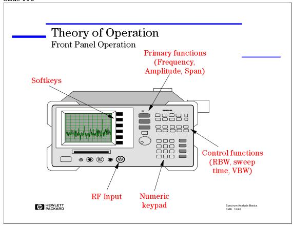
Before we move on, its important to know what we can control on the analyzer via the front panel keys.
