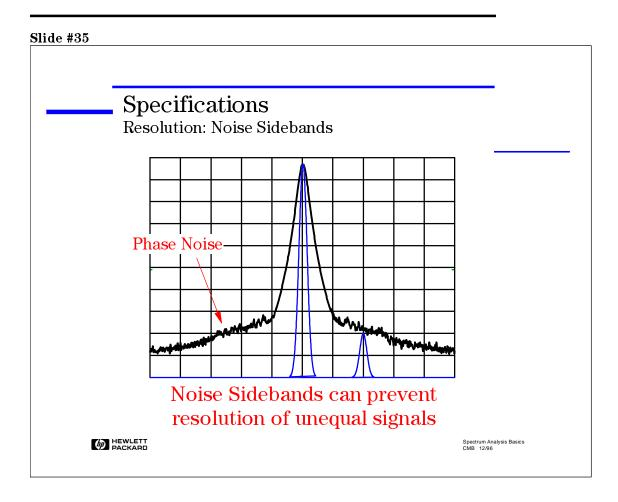
The remaining instability appears as at the base of the signal response. This noise can mask close-in (to a carrier), low-level signals that we might otherwise be able to see if we were only to consider bandwidth and selectivity. These noise sidebands affect resolution of close-in, low-level signals.
