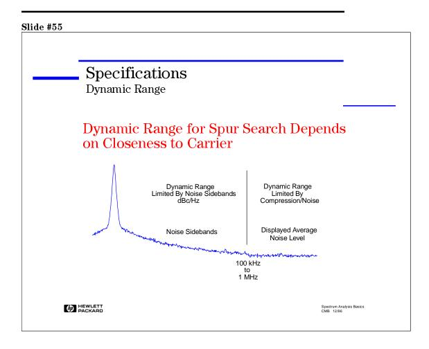
The final factor in dynamic range is the phase noise, or noise sidebands, on our spectrum analyzer LO.
