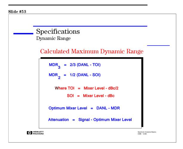
Maximum dynamic range is easy to calculate, as shown on the slide.
