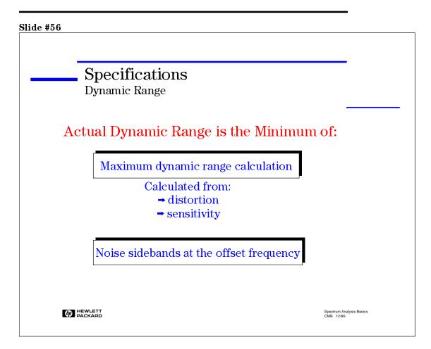
We have seen that the dynamic range of a spectrum analyzer is limited by three factors: the broadband noise floor (sensitivity) of the system, the distortion performance of the input mixer, and the phase noise of the local oscillator. The first two factors are used to calculate maximum dynamic range. Therefore, actual dynamic range is the minimum of 1) the MDR calculation and 2) the noise sidebands.
