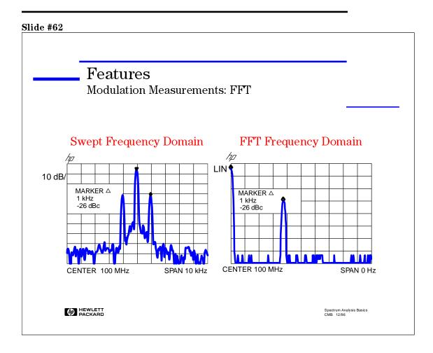
Another common measurement made on an AM signal (besides determining the modulation frequency) is modulation index, which tells us the degree of modulation (0 to 100%).
