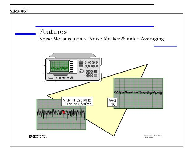
When making measurements on noise, there are a couple of features on a spectrum analyzer that can make the measurements easier and more accurate.
