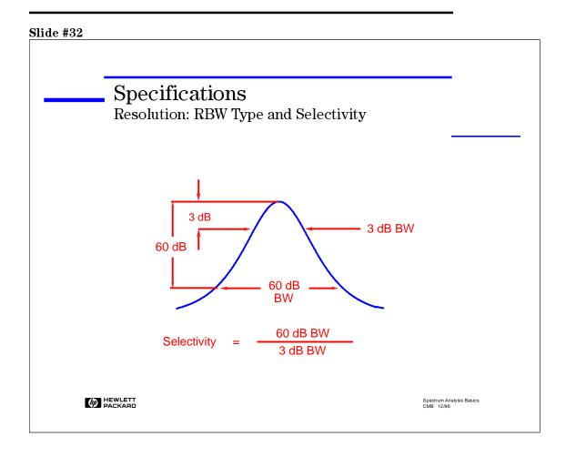
Selectivity is the important characteristic for determining the resolvability of <u>unequal</u> amplitude signals. Selectivity is the ratio of the 60 dB to 3 dB filter bandwidth. Typical selectivities range from 11:1 to 15:1 for analog filters, and 5:1 for digital filters.
