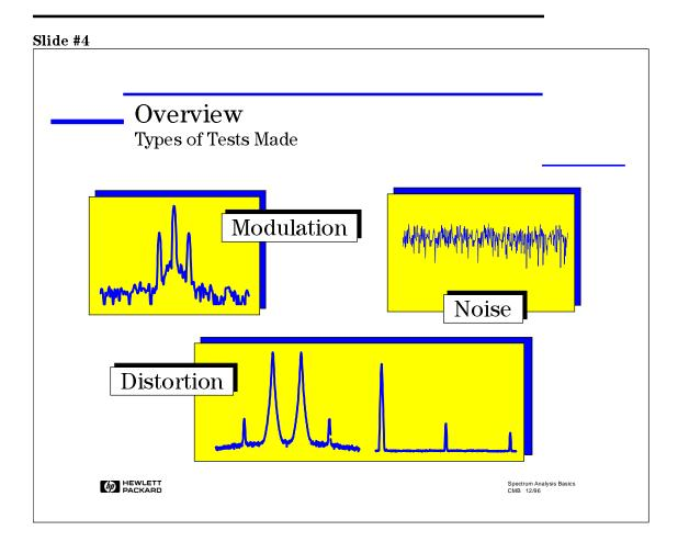
The most common spectrum analyzer measurements are: modulation, distortion, and noise.
