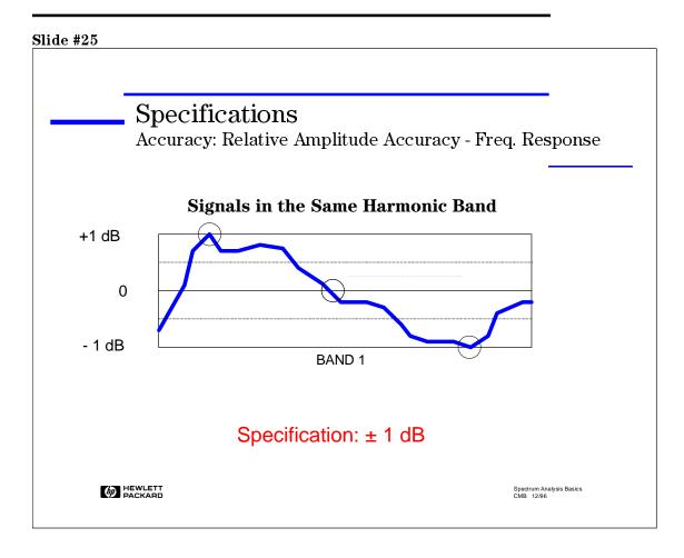
The frequency response, or flatness of the spectrum analyzer, also plays a part in relative amplitude uncertainties and is frequency-range dependent. A low-frequency RF analyzer might have a frequency response of  $\pm 0.5$  dB. On the other hand, a microwave spectrum analyzer tuning in the 20 GHz range could well have a frequency response in excess of  $\pm 4$  dB.
