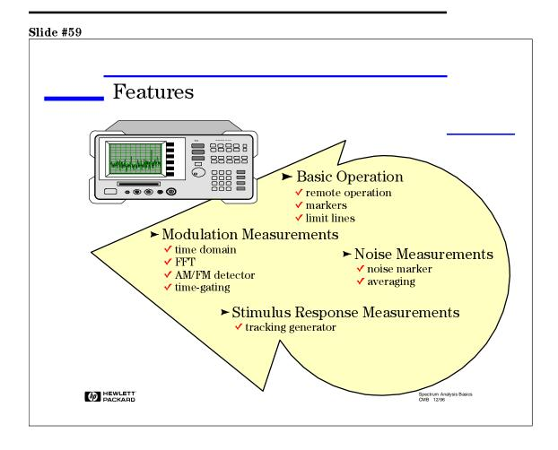
The features are categorized into application areas, in order to better describe their function. The first group, under Basic Operation, are some of the key features that enhance the use of the analyzer for any application. The others refer to a specific application, although the feature is not necessarily used *only* in that application.
