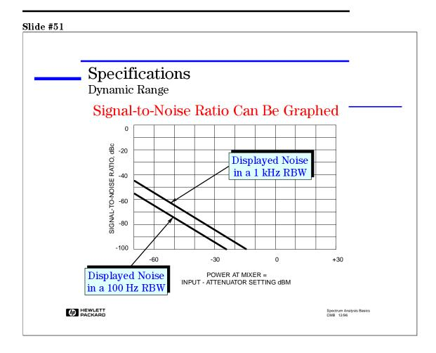
On page 48, we plotted the signal-to-distortion curves. This graph is actually called a dynamic range graph, and just as we plotted distortion products as a function of mixer power, we can also plot *signal-to-noise ratio* (SNR) as a function of mixer power.
