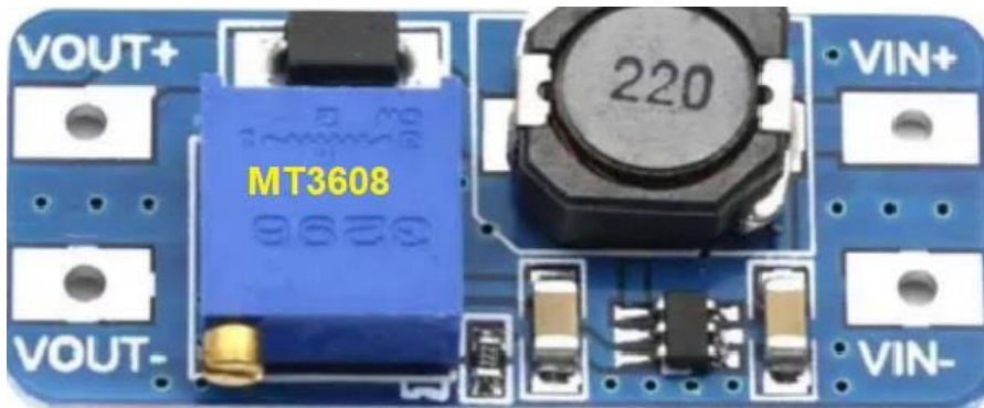
Fig. 2 – Conversor DC-CD step up MT 3608
