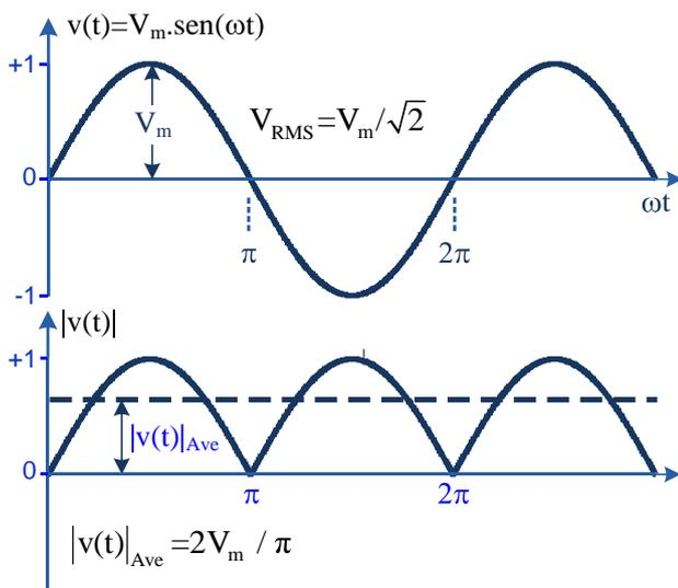
Figura 5 - Fator 1.11 dos multímetros Average Sensing.
